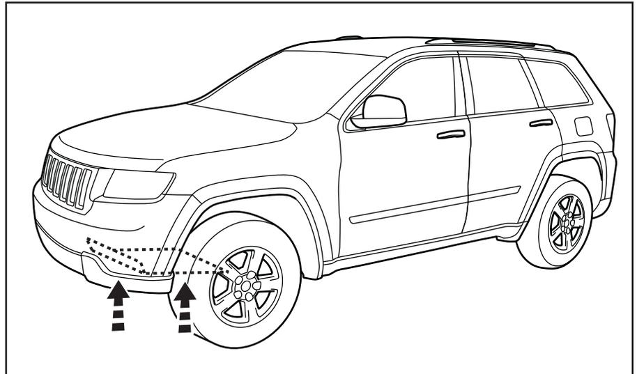
2. Bolt Front Skid Plate into position as shown using (4) 13mm bolts and (4) clip nuts provided. Tighten to 19 Nm (14 ft. lbs.)
