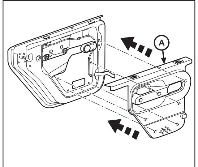
3. Install 2 Phillips screws - long (C) through upper holes in door trim panel (A). Tighten with phillips screwdriver.
