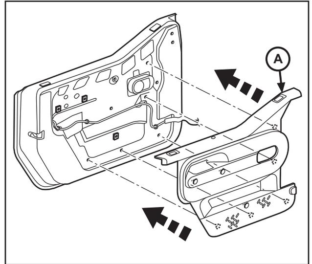
3. Install 2 Phillips screws - long (D) through upper holes in door trim panel (A). Tighten with phillips screwdriver.
