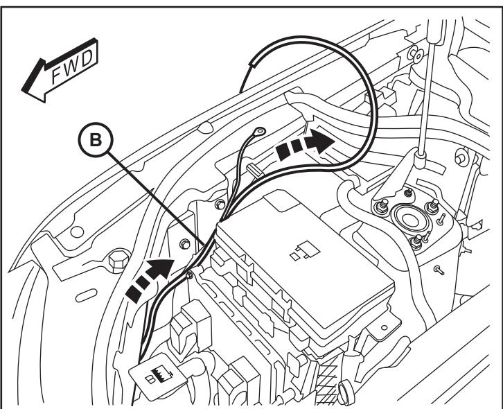
9. Inside the fender edge, remove the existing long hex nut. Position the ground ring terminal from the switch harness onto the stud (B) and reattach the nut to secure.
