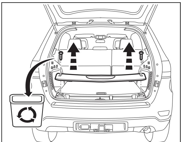
30. Remove the cargo deck cover panel from the vehicle.
