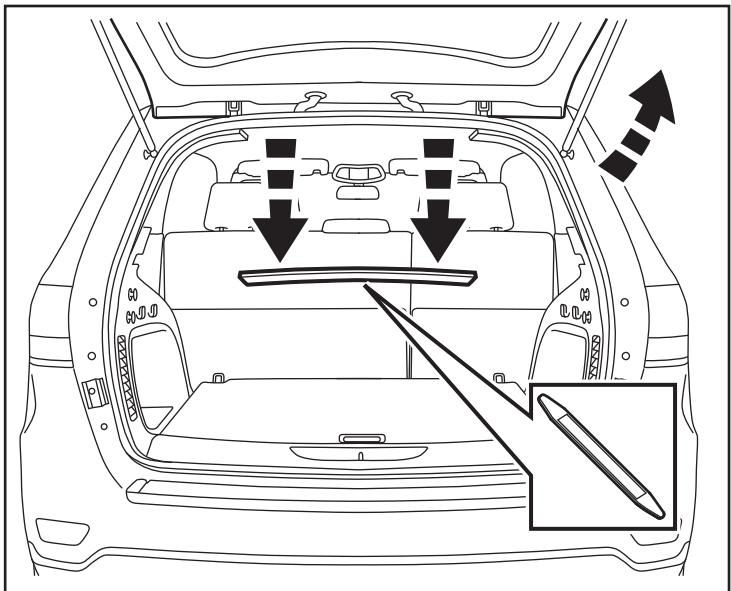
29. Remove two (2) fasteners from the bottom scuff panel. Remove the panel from the vehicle.
