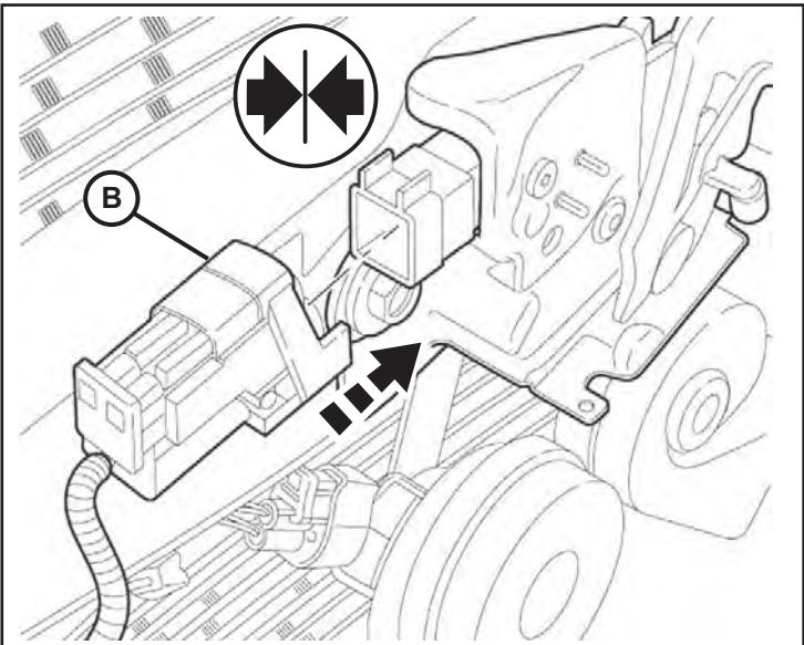
7. Carefully pry back the radiator cover panel. Route the switch harness (B) over towards the passenger side along the existing vehicle harness. Feed the switch harness under the upper cross member and out next to the washer fluid bottle. Secure with cable ties (E).
