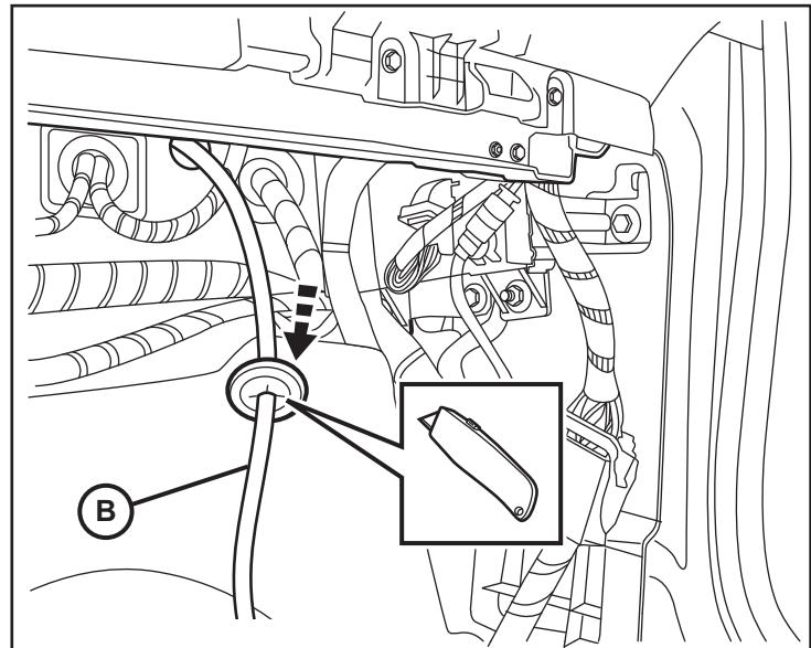
22. Locate the BCM up under the glovebox on the outer wall of the passenger side footwell. The top left connector (**D3806A**) will need to be accessed for the new harness connector. To have enough working slack in the BCM wiring harness, remove ALL the connectors from the BCM and carefully pull the harness down.
