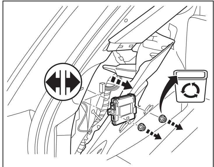
33. Plug the Antenna Module cable (D) into the new RF Hub module (C).
