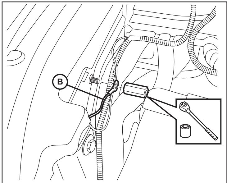
10. Route the switch harness (B) under the rear cross member and out near the positive battery terminal.
