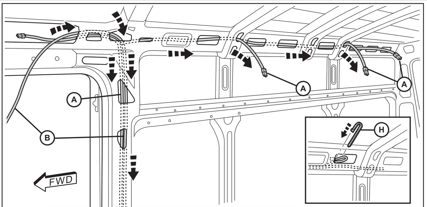
NOTE: TWO LIGHT BARS ARE PROVIDED IN THE KIT. HARNESS COMES WITH FOUR LAMP CONNECTORS. LIGHT BAR MOUNTING POSITIONS ARE OPTIONAL. EXTRA LIGHT BARS CAN BE ADDED TO HARNESS. **BUNDLE AND STOW UNUSED CONNECTORS ON THE HARNESS.**
