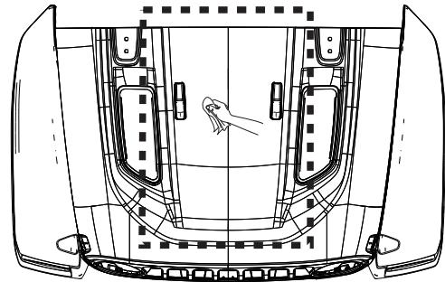
Align Template To Sheet Metal Edges
