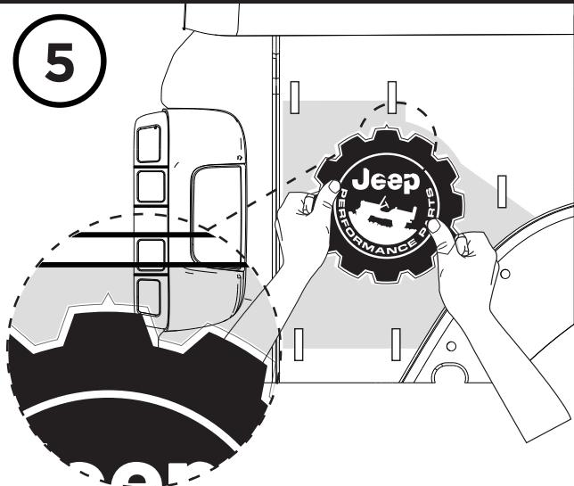
Align Decal To Installation Template Using Center Notch
